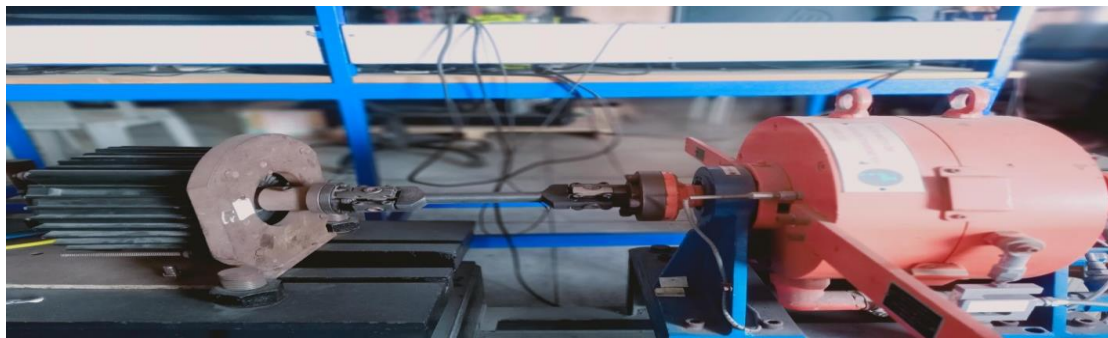
Fig. 5 Experimental Setup for torque measurement
